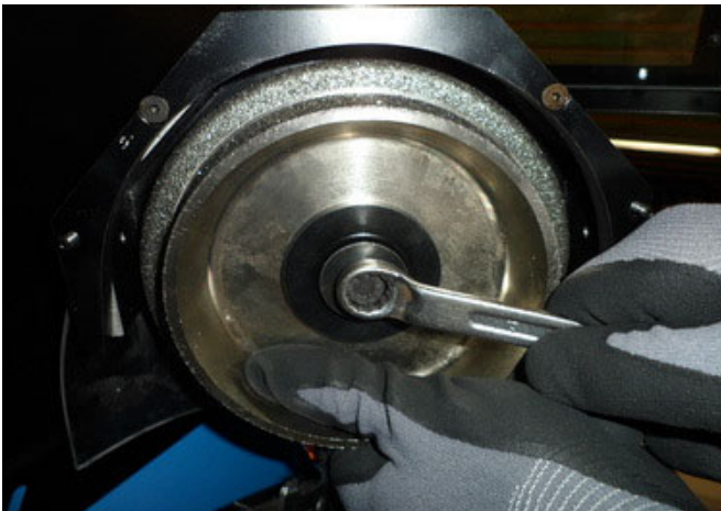
Image 35. Changing the grinding wheel
