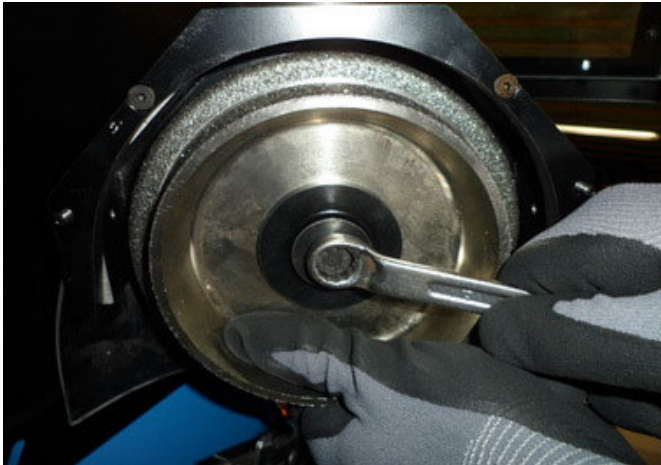
Image 41. Changing the grinding wheel
