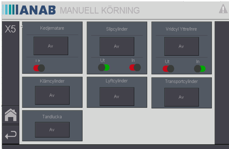
Image 30. Setting for manual operation
