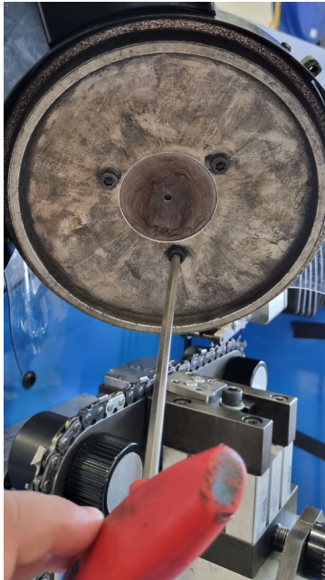
Image 42. Changing the grinding wheel
